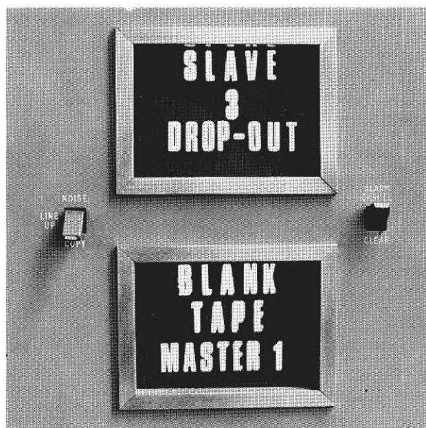
Fig. 5 Close-up of visual display unit showing typical fault display
